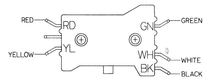
The above procedure can be used on all one speed washers except for the 132 and 132S. Below is the wire harness hookup for the 132 and 132S.
